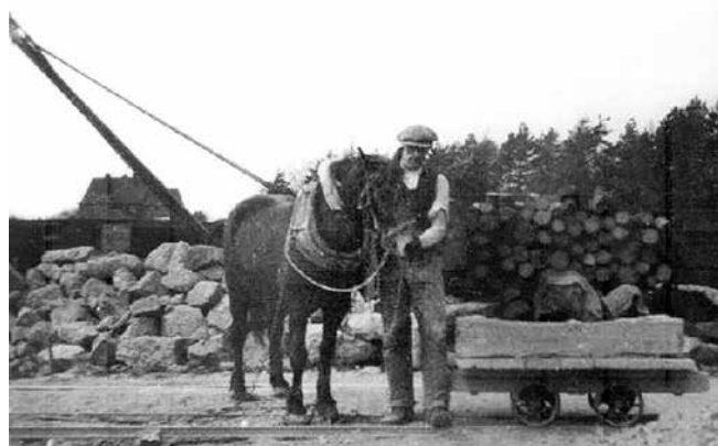
Colley Hill mine hearthstone factory. Lumps of stone from the mine can be seen in a stockpile. The large lumps were broken into smaller pieces and then ground to powder to be moulded into small blocks. Completed blocks are seen here set out to dry. A stockpile of pit props is seen on the right. The large stone slab on a trolley may have been intended for use as a hearth, rather than for whitening a stone hearth
